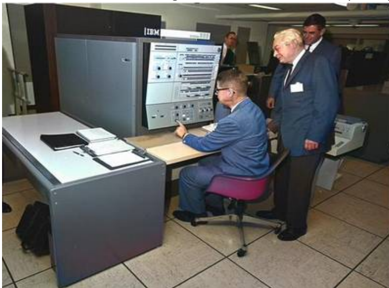
IBM/360 from 1964 was a series of computers and peripherals, all compatible with each other. It used tightly packed transistors. A great step forward. Here's a basic unit.
